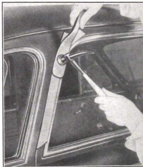
Fig. 1-94. Spring-hammering door flange to make it fit flush with adjacent body panel. Tape the flange before spring-hammering.
