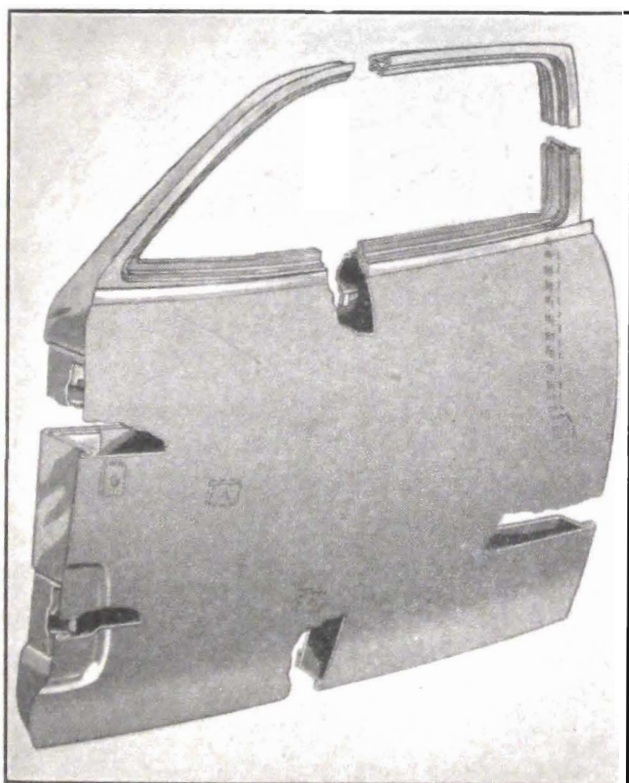
Fig. 1-39. Cutaway View—Front Door—Series 50-70
