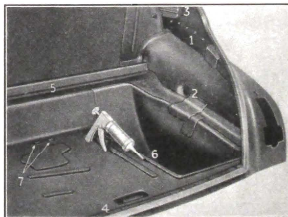
Fig. 1-122. Rear compartment floor and side wall construction, showing where to inspect and seal for water leaks.
