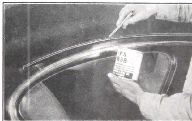
Fig. 1-116. Water sealing at the spot-welded junction of the roof panel and drip molding.
