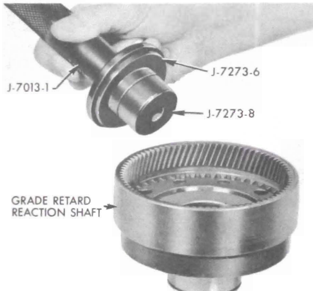
238D. Install new grade retard reaction shaft front bushing using J-7013-1 Handle and J-7273-6-8. (Counterbore on 6 toward handle.)
