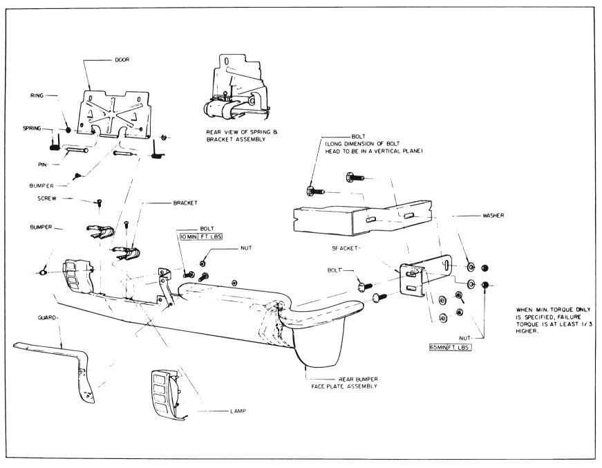
Figure 12-17—Rear Bumper Installation—4700 Series
