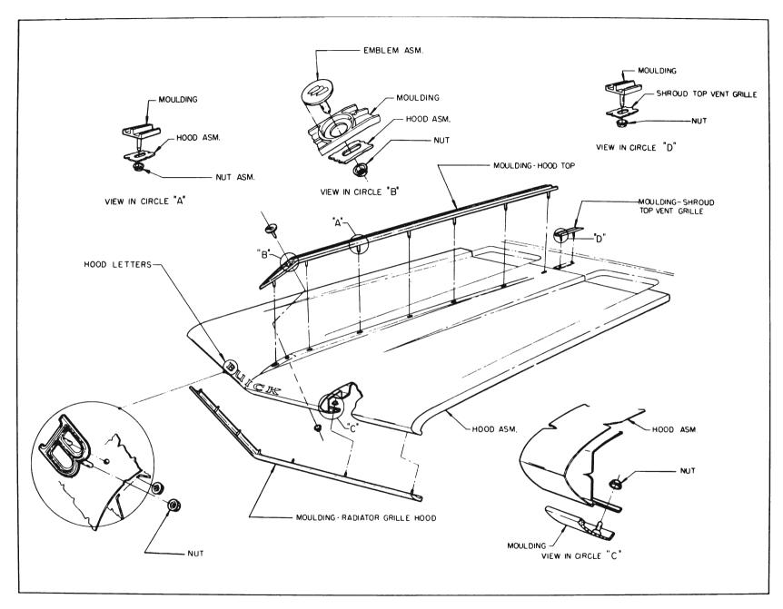
Figure 12-16-Hood Installation-4700 Series
