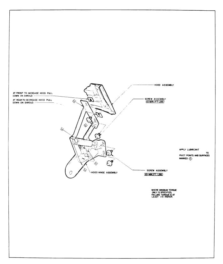
Figure 12-7-Hood & Hood Hinge Assembly-4400-4600-4800 Series
