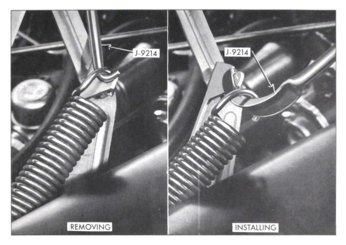
Figure 12-6—Removing and Installing Hood Hinge Spring
