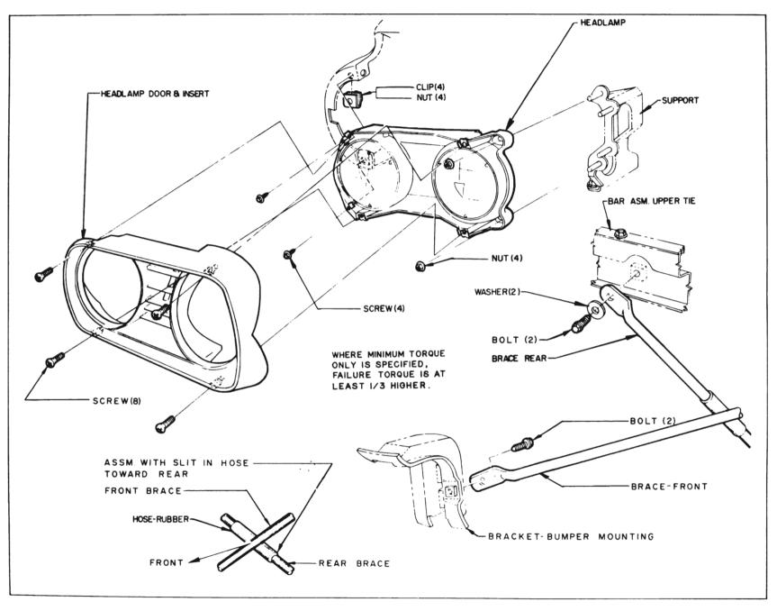
Figure 12-13-Headlight Installation-4400-4600-4800 Series
