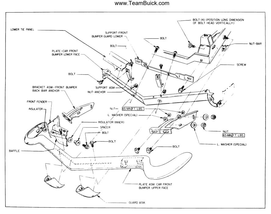
Figure 12-9-Front Bumper Assembly-4700 Series
