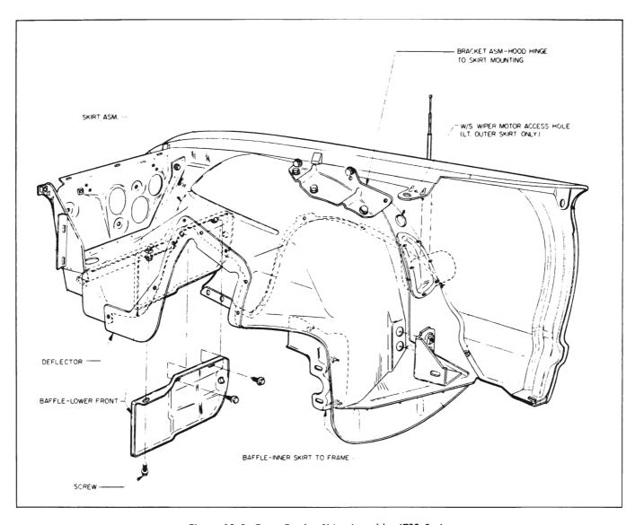
Figure 12-2-Front Fender Skirt Assembly-4700 Series
