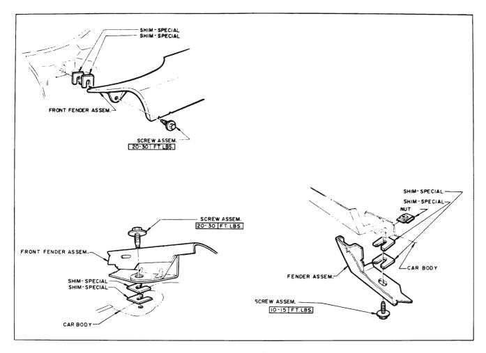
Figure 12-5-Front Fender Adjustment
