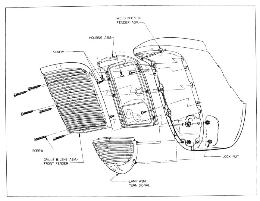
Figure 12-12—Parking Lamp, Cornering Light, & Directional Signal Grille Assembly—4700 Series
