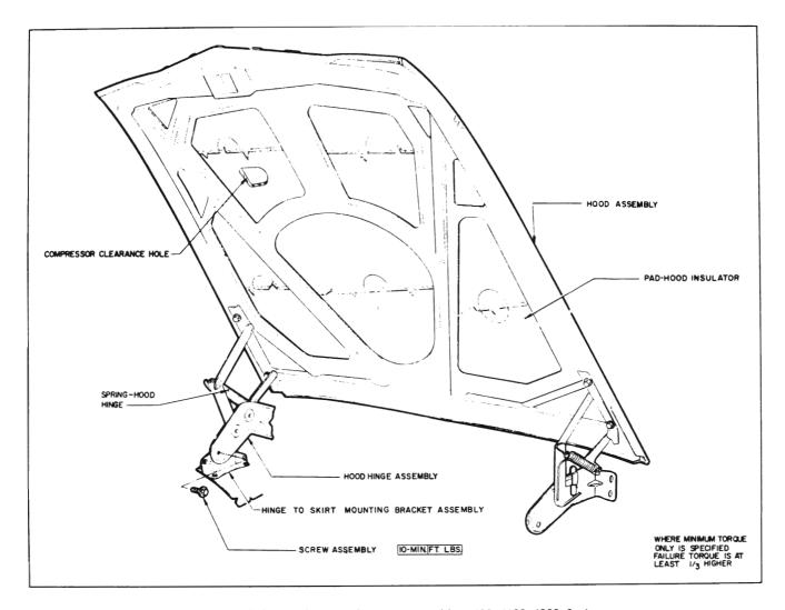
Figure 12-3-Hood & Hood Hinge Assembly-4400-4600-4800 Series
