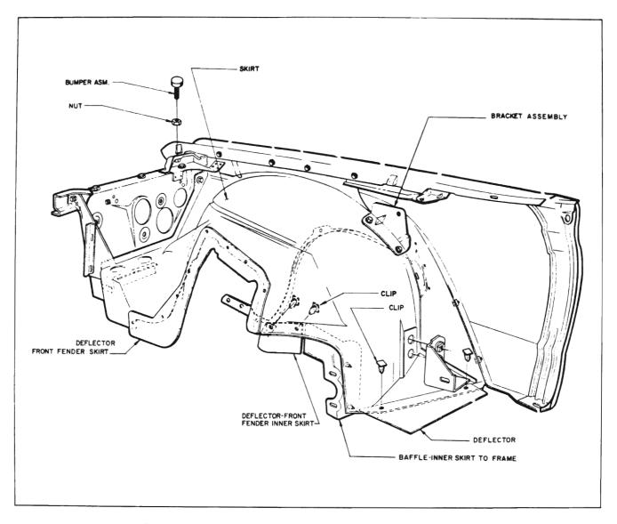
Figure 12-1—Front Fender Skirt Assembly-4400-4600 and 4800 Series
