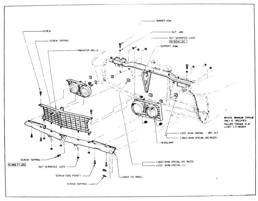
Figure 12-14-Radiator, Grille, & Headlamp Installation-4700 Series
