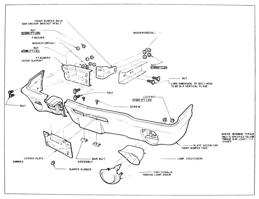
Figure 12-10-Front Bumper Assembly-4400-4600-4800 Series
