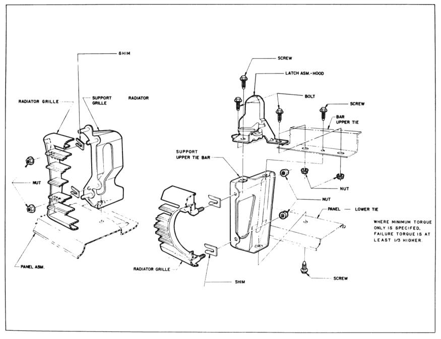
Figure 12-11-Radiator, Grille Assembly-4400-4600-4800 Series
