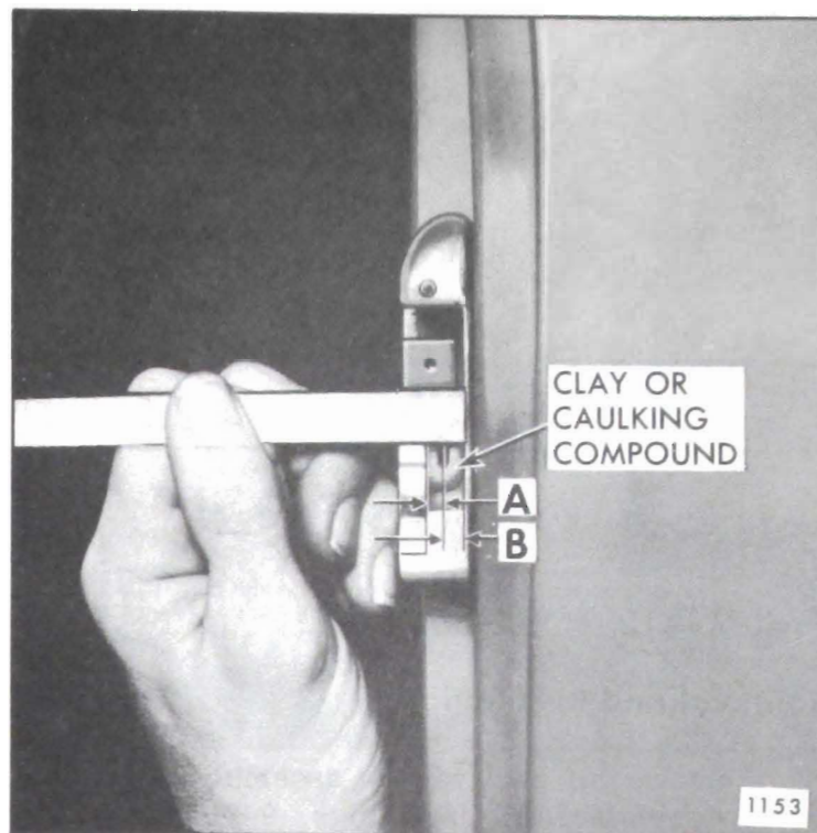
Fig. 9-46—Tail Gate Lock Striker Caulking Check
