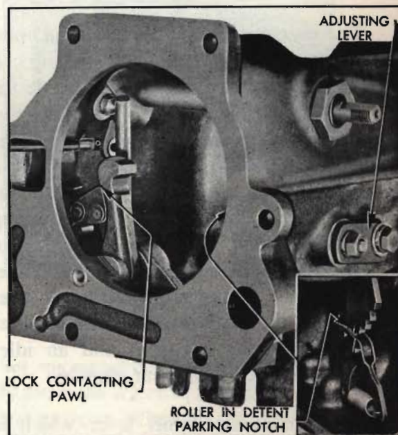
Fig. 5. Shift detent adjustment
