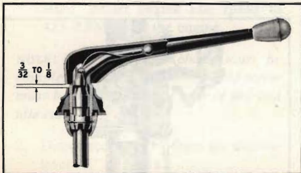
Fig. 8. Steering column upper support to control lever clearance
