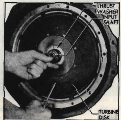
Fig. 23. Removing twin turbine assembly
