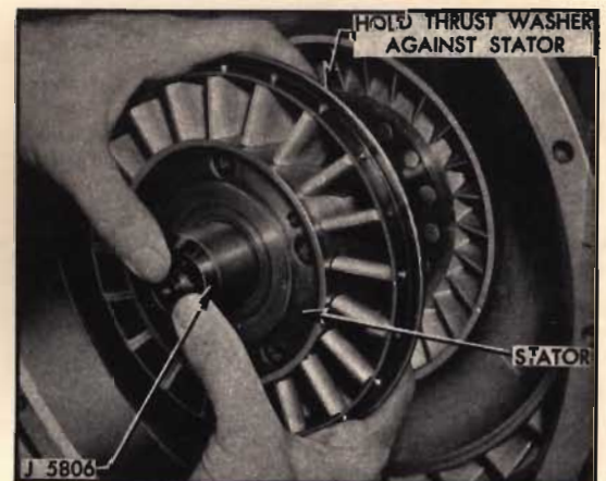
Fig. 3. Removing stator assembly
