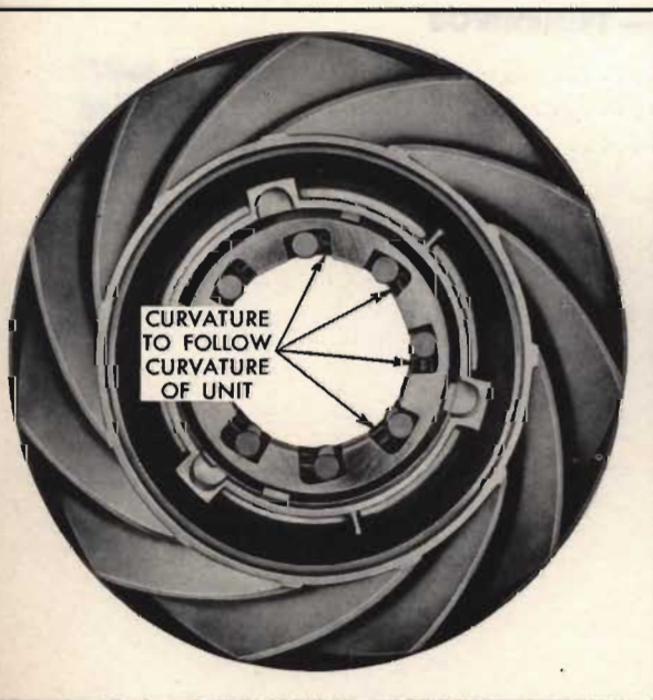
Fig. 24. Curvature of spring retainers
