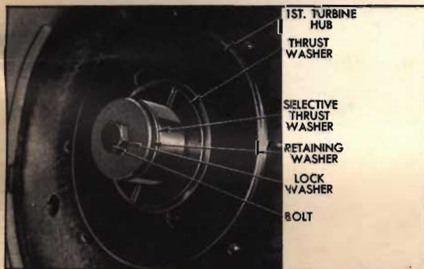
Fig. 1. Turbine retaining washer and thrust washer
