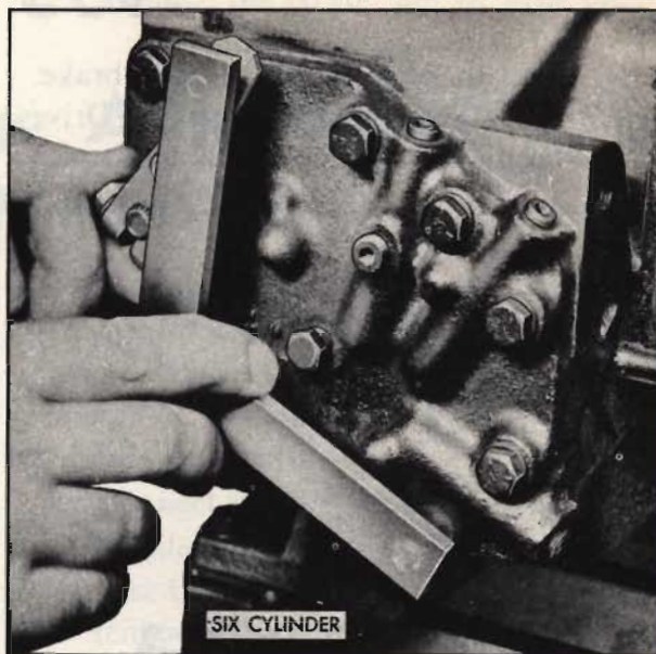
Fig. 2. Use of outer throttle valve lever gauge six cylinder
