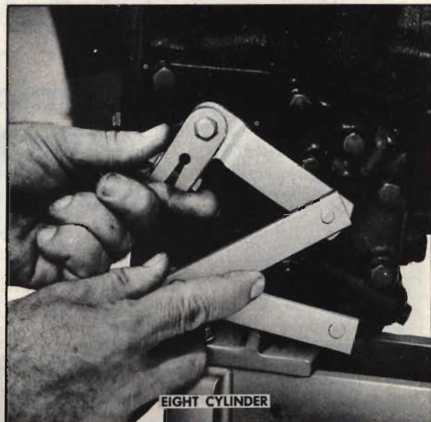
Fig. 6. Use of outer throttle valve lever gauge eight cylinder
