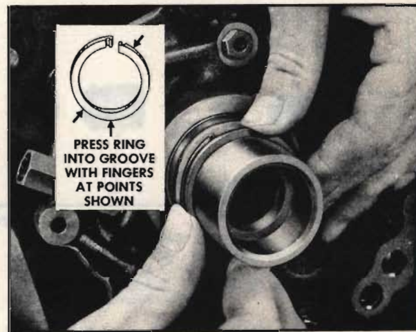
Fig. 3. Installing oil seal rings
