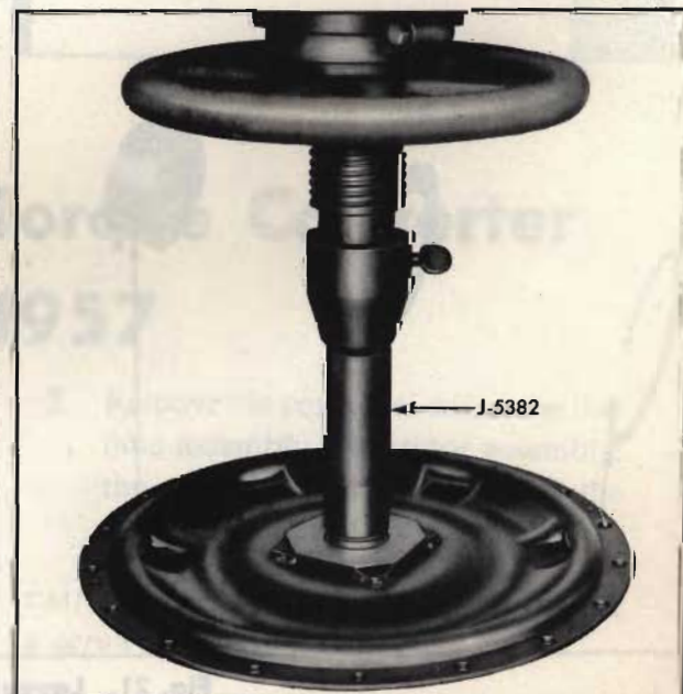
Fig. 23. Replacing converter cover bushing
