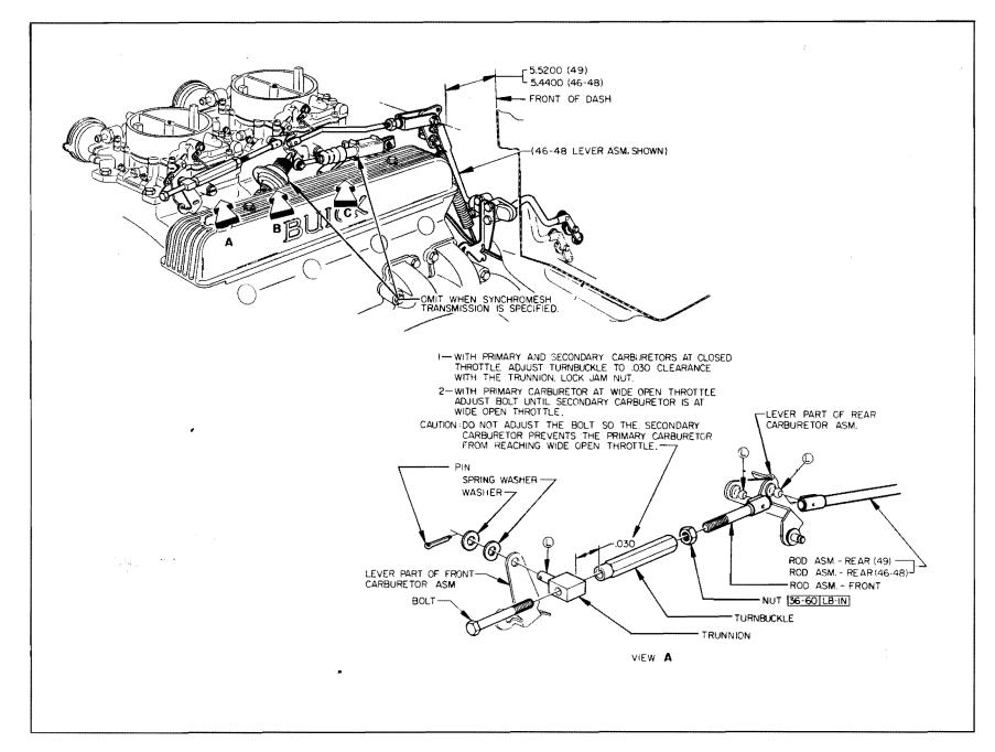
Figure 3-83—Throttle Control Information - Dual 4-Barrel
