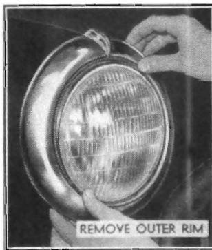
Fig. 12-65 Swing rim out at bottom and lift upward to disengage lug at top of rim
