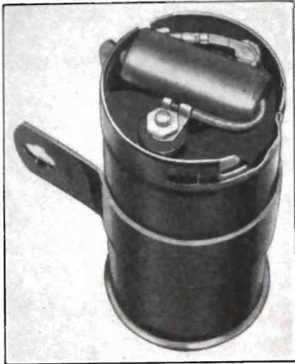
Fig. 12-35. Condenser Installation for Radio Jobs
