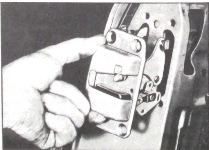
Figure 13-11—Door Lock Removal—1949 Series 50-70
