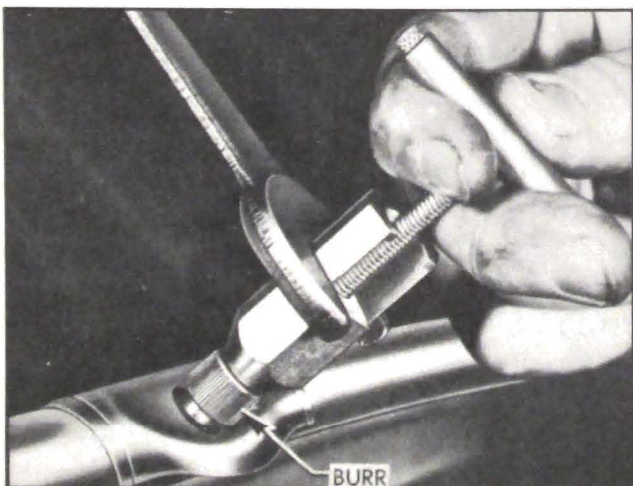
Figure 13-27—Installing Driving Burr on Transmission Shaft
