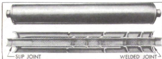
Figure 3-8—Muffler—Sectional View
