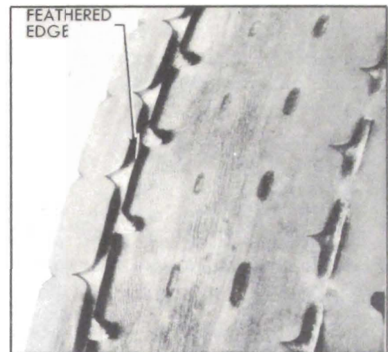
Figure 6-11—Toe-in or Toe-out Tread Wear
