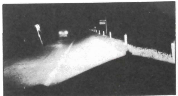
Figure 10-85—Light Distribution with Lower Headlight Beam
