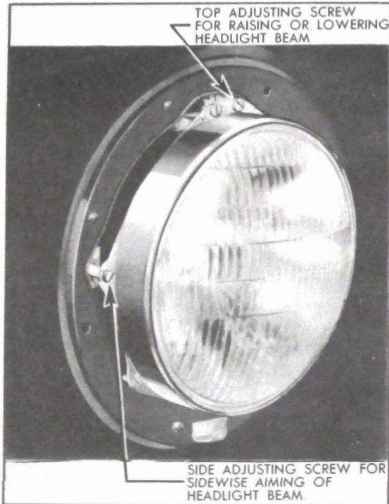
Figure 10-88—Headlamp Aiming Adjustments
