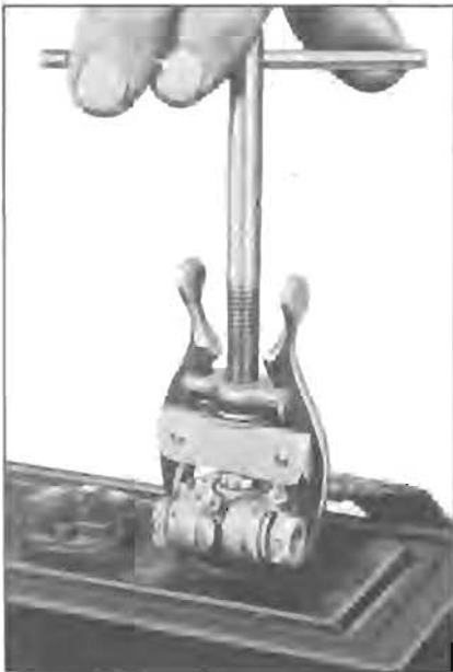
Figure 10-9—Removing Corroded Terminal with Puller
