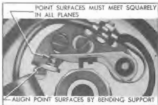
Figure 10-67—Contact Point Alignment
