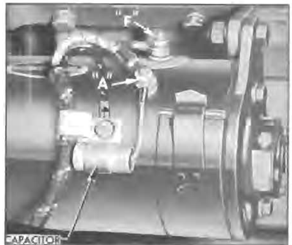
Figure 11-13—Capacitor Mounted on Generator
