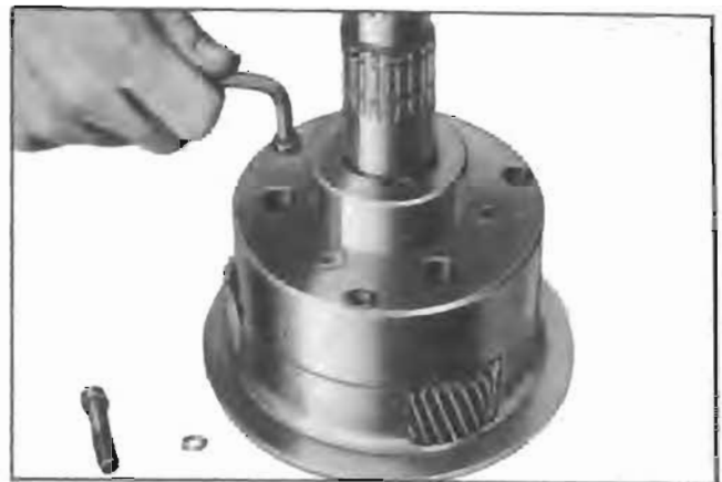
Figure 4-123—Removing Planet Carrier Screws
