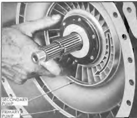
Figure 4-77—Checking Secondary Pump Free Wheeling Clutch
