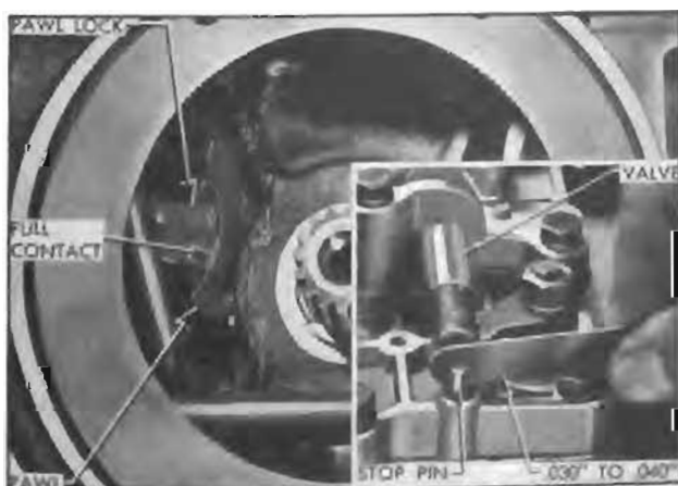
Figure 4-146—Control Valve Linkage Adjustments
