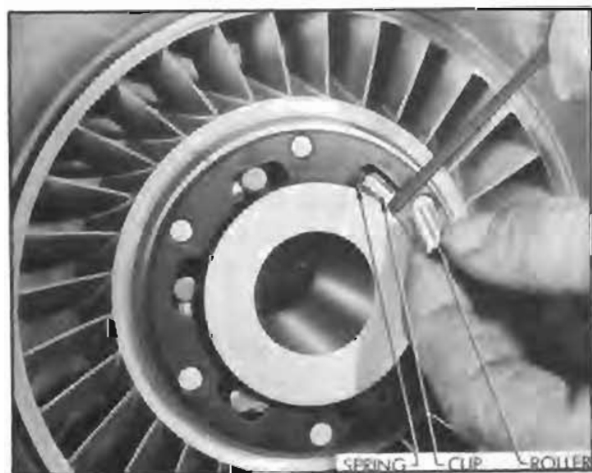
Figure 4-96—Installing Free Wheel Rollers in Pump
