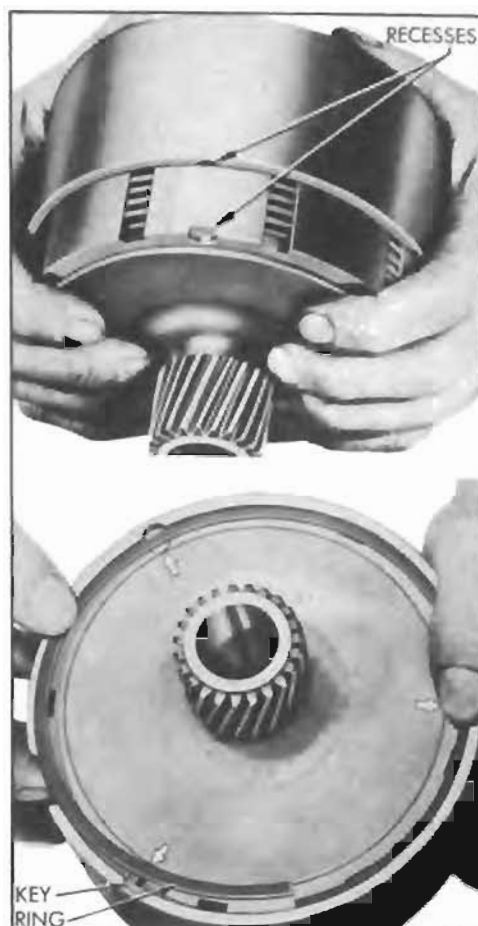
Figure 4-117—Installing Drum Over the Reaction Gear Flange
