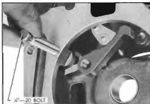
Figure 4-120—Removing Lock Pawl Shaft
