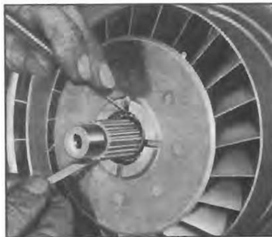
Figure 4-150—Installing Reaction Shaft Retaining Ring
