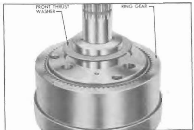
Figure 4-132—Installation of Front Thrust Washer
