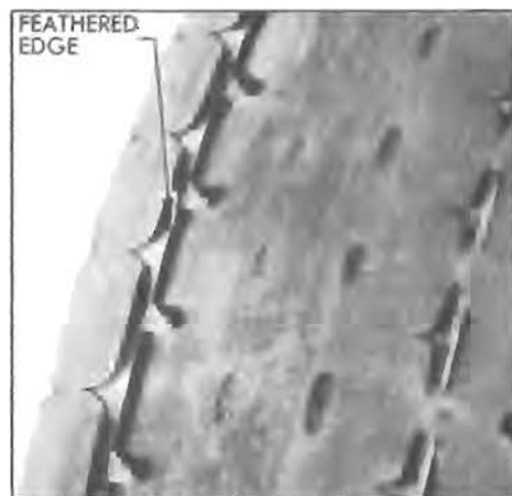
Figure 6-11—Toe-in or Toe-out Tread Wear
