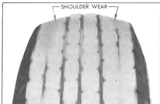
Figure 6-9—Underinflation Tread Wear
