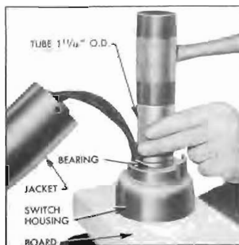
Figure 7-10—Installing Control Shaft Bearing
