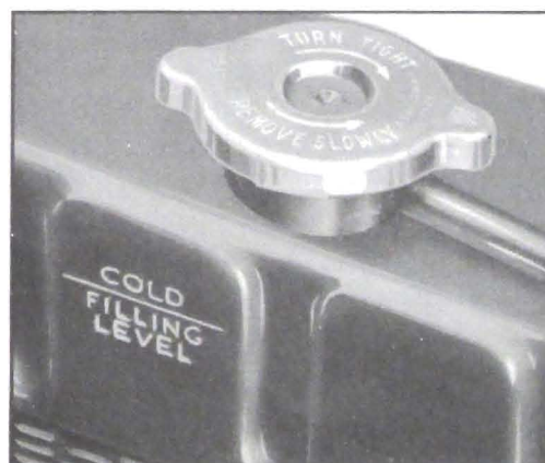
Figure 1-6—Radiator Filling Level—Cold
