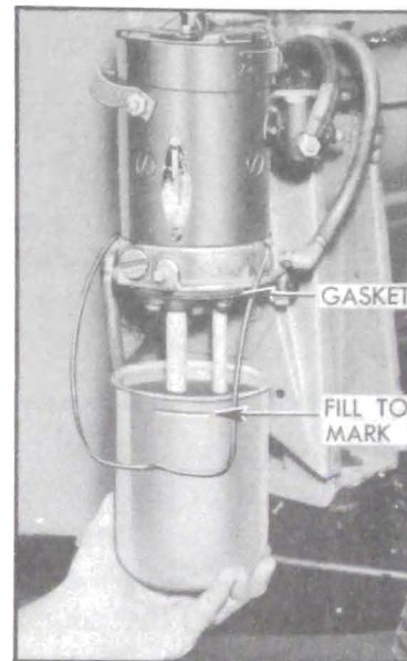
Figure 1-17—Filling H-L Power Unit Reservoir
