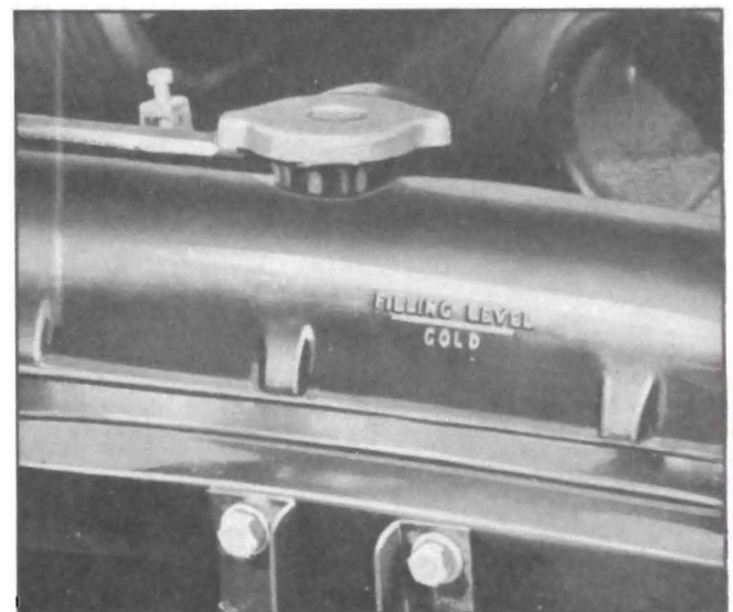
Figure 1-4—Radiator Filling Level—Cold
