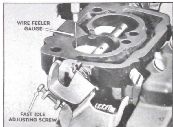
Figure 3-30—Adjusting Fast Idle Speed (on Bench)
