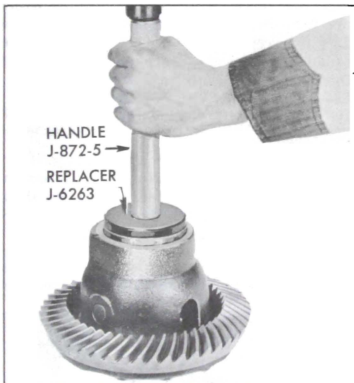
Figure 6-31—Installing Differential Bearing Outer Race
