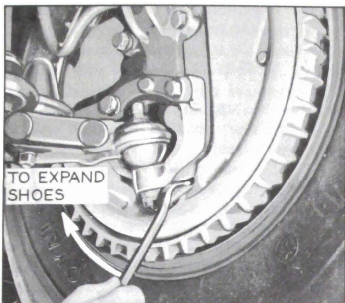
Figure 9-8—Expanding Brake Shoes
