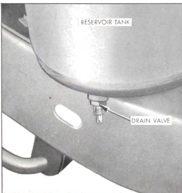
Figure 1-10—Air Ride Air Reservoir Tank Drain Valve
