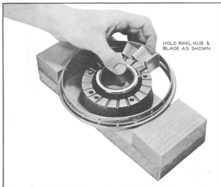
Figure 5-53—Inserting Stator Blades in Carrier
