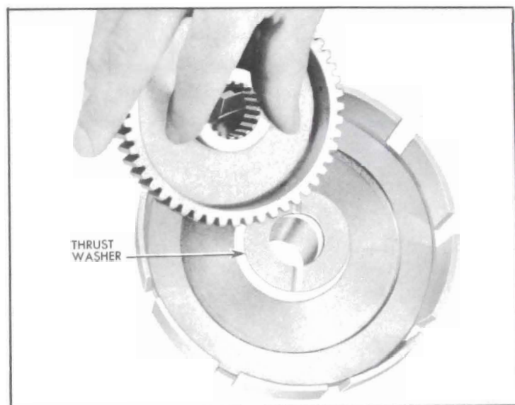
Figure 5-76—Installing Thrust Washer and Clutch Hub in Reaction Gear
