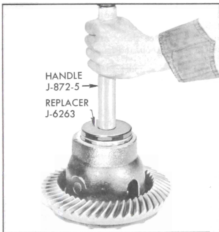
Figure 6-31—Installing Differential Bearing Outer Race
