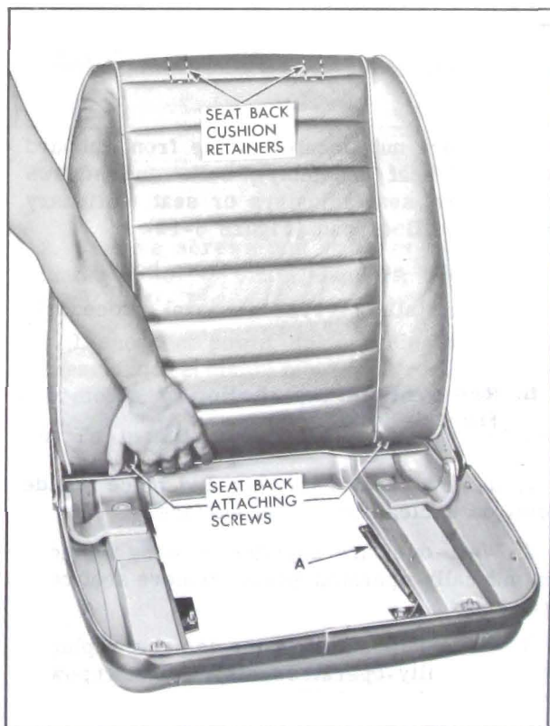
Figure 5-11—Removal of Bucket Type Seat Back Cushion
