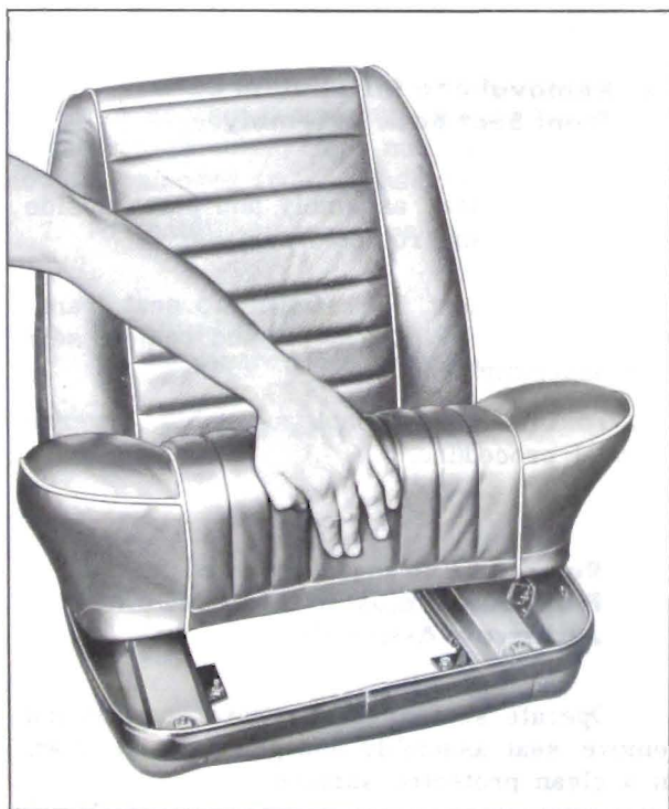
Figure 5-10—Removal of Bucket Type Seat Cushion
