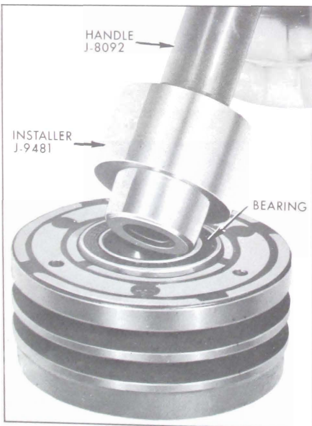
Figure 11-84—Installing Pulley Bearing
