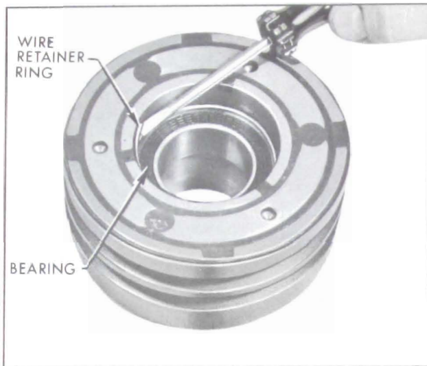
Figure 11-83—Removing Bearing Retainer Wire
