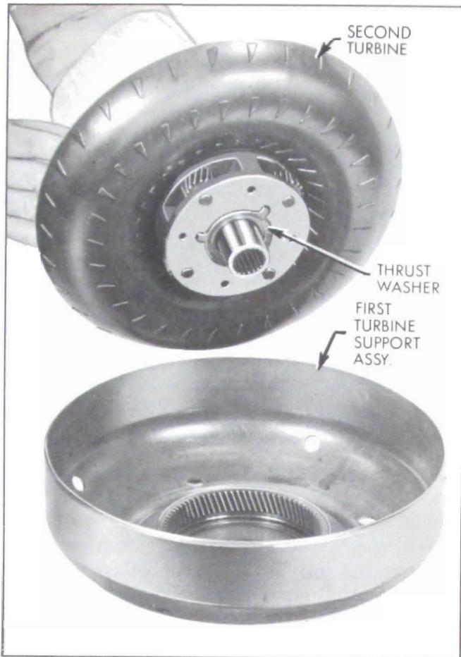
Figure 5-63—Installing Second Turbine in First Turbine Support
