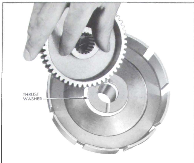
Figure 5-91—Installing Thrust Washer and Clutch Hub in Reaction Gear
