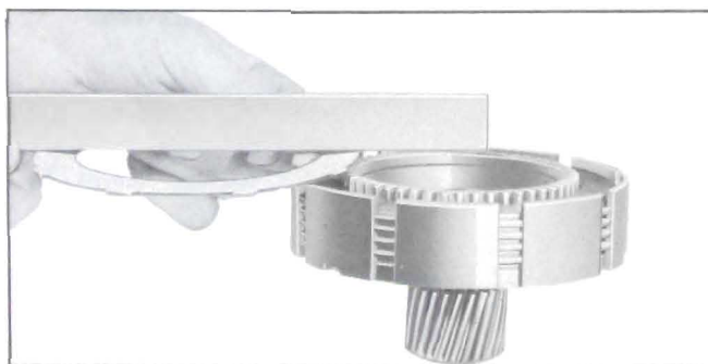
Figure 5-92—Checking "Dished" Side of Externally Splined Clutch Plate
