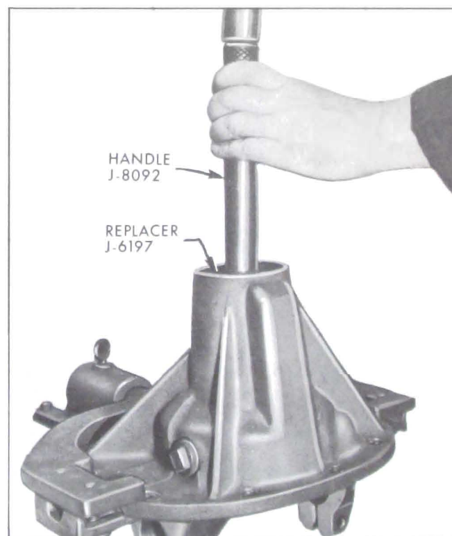
Figure 6-16—Installing Front Pinion Bearing Outer Race
