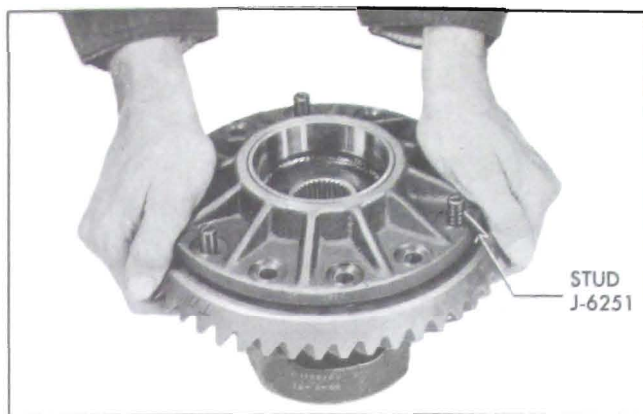
Figure 6-28—Installing Ring Gear on Differential Case
