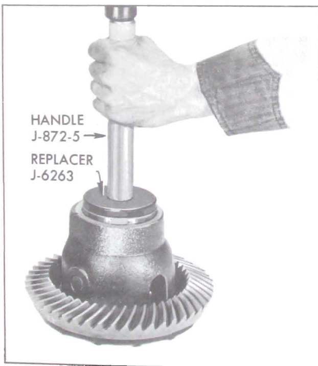
Figure 6-27—Installing Differential Bearing Outer Race
