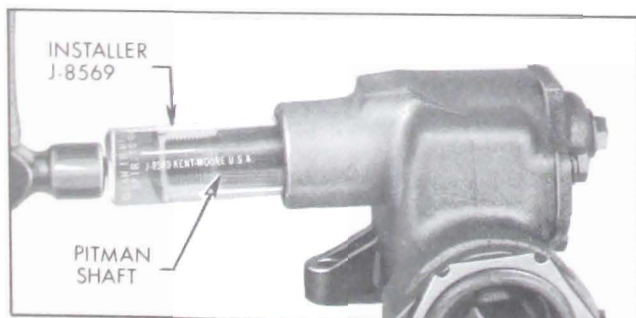
Figure 8-11—Installing Pitman Shaft Seal
