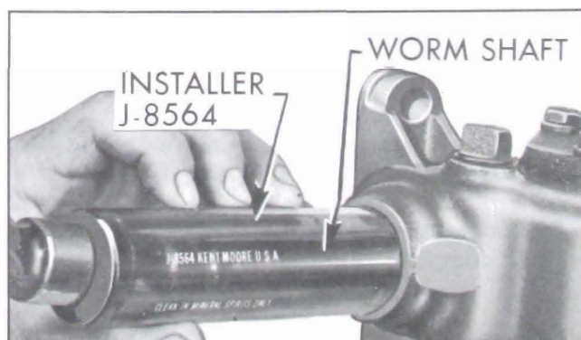
Figure 8-12—Installing Worm Shaft Seal
