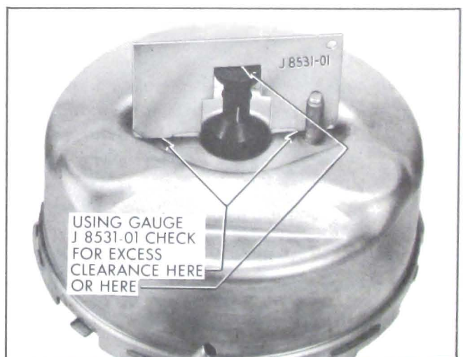
Figure 9-26—Gauging Master Cylinder Piston
