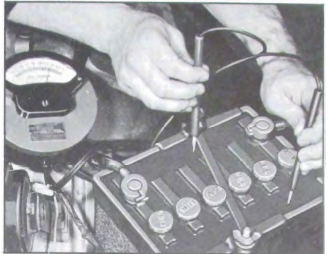
Figure 10-3--Light Load Test
