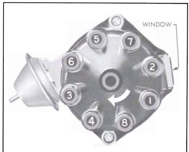
Figure 10-37—Installing Spark Plug Wires in Cap (V-8 Engine)
