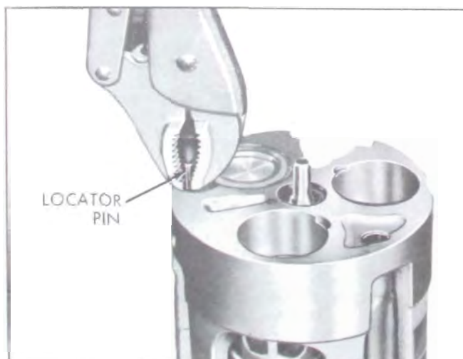
Figure 11-82—Removing Locator Pin
