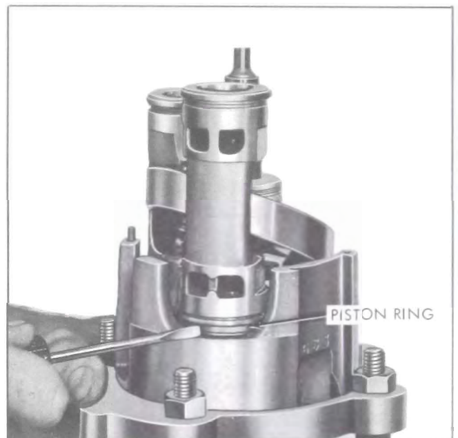
Figure 11-76—Compressing Front Piston Ring
