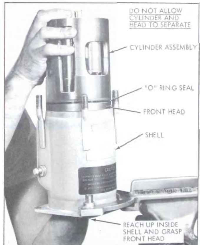
Figure 11-87—Inserting Cylinder Assembly in Shell
