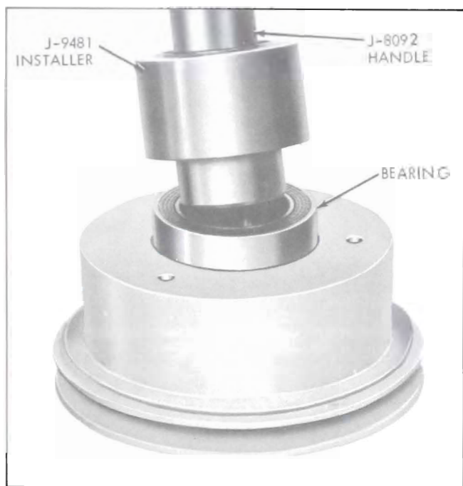
Figure 11-46—Installing Pulley Bearing
