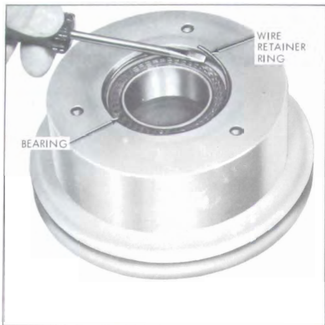
Figure 11-45—Removing Bearing Retainer Wire
