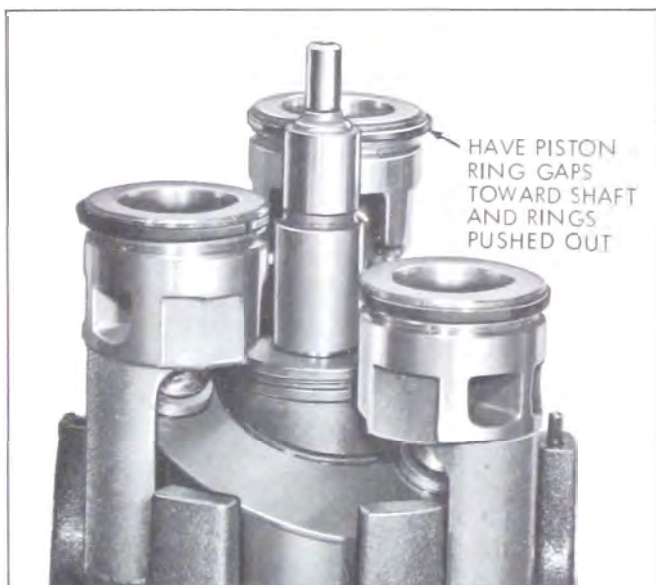
Figure 11-78—Front Cylinder Half Assembly
