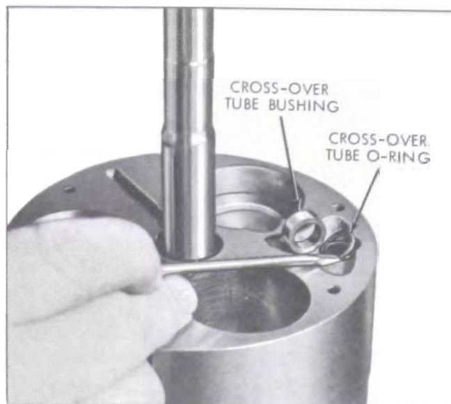
Figure 11-83—Installing Crossover Tube O-Ring
