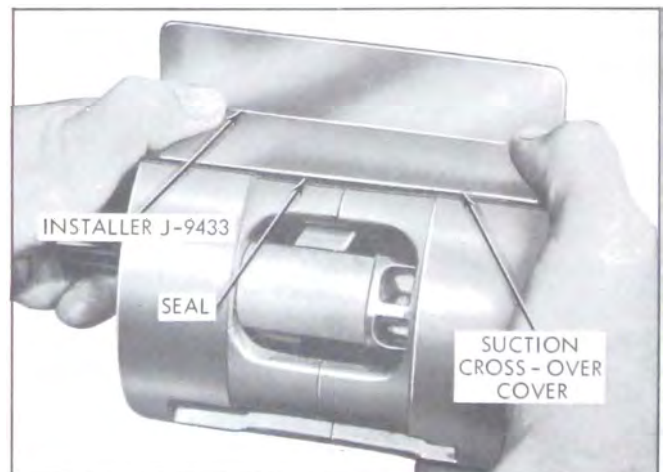
Figure 11-80—Installing Suction Cross over Cover and Seal
