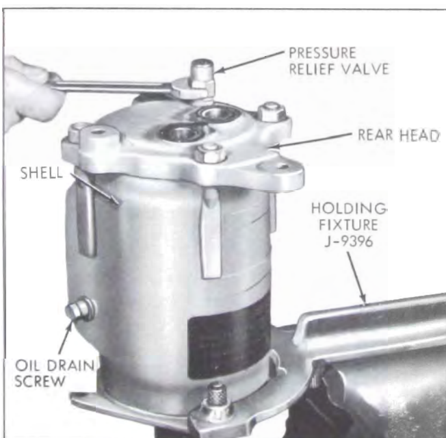
Figure 11-54—Removing Pressure Relief Valve
