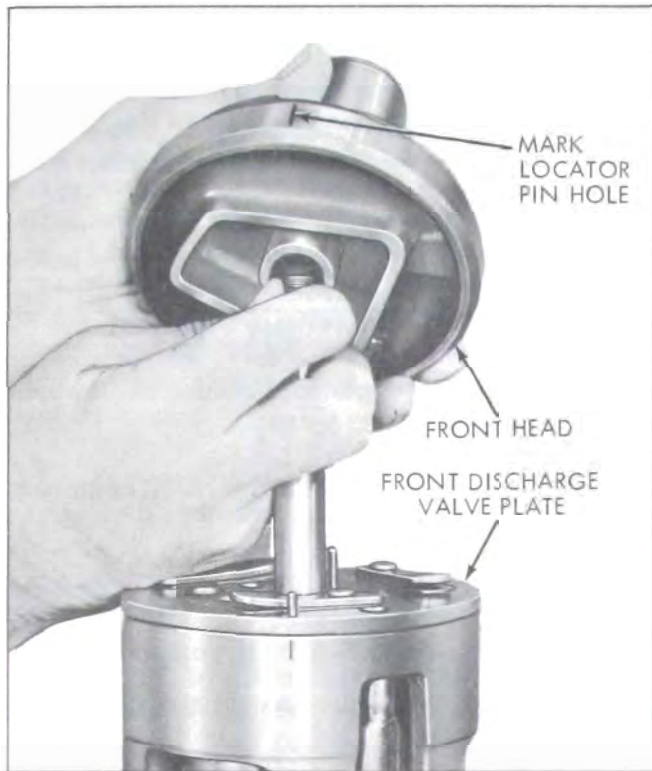
Figure 11-85—Placing Front Head on Cylinder Assembly
