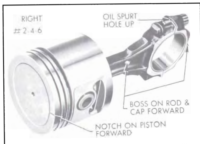
Figure 2-59—V-6 Right Bank Piston and Rod Assembly
