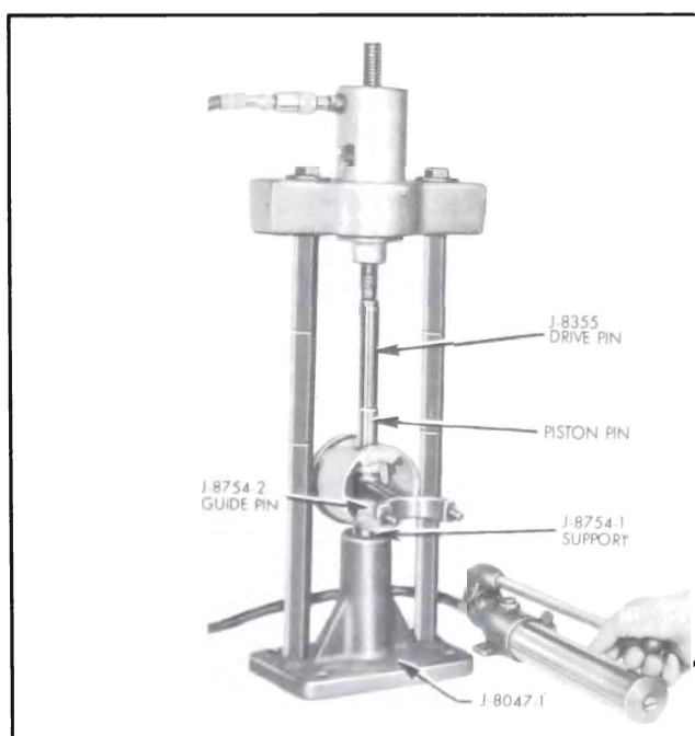
Figure 2-55—Installing Piston Pin
