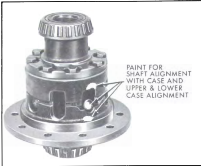
Figure 6-51—Alignment Marks
