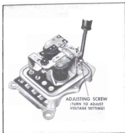
Figure 10-26—Adjusting Voltage Regulator Setting
