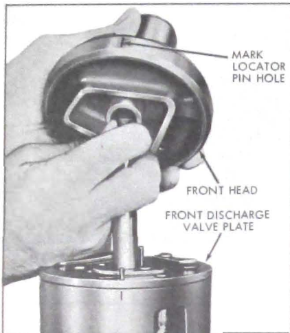
Figure 11-144—Placing Front Head On Cylinder Assembly
