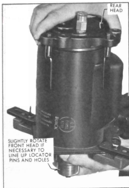
Figure 11-148—Installing Rear Head
