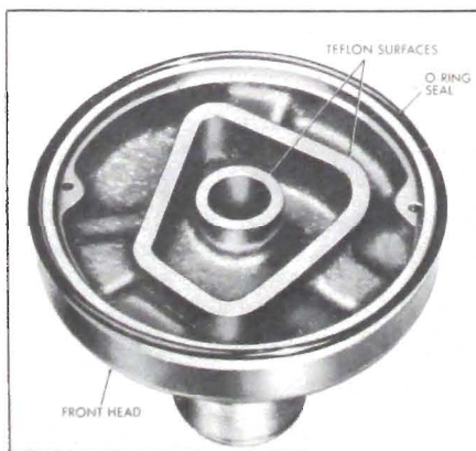
Figure 11-119—Front Head Teflon Sealing Surfaces
