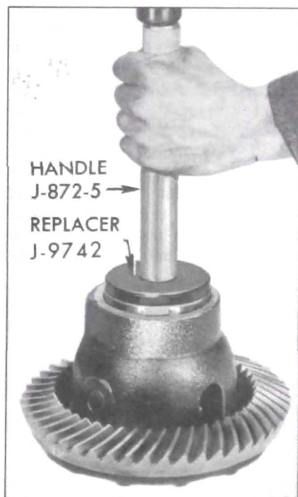
Figure 6-30—Installing Differential Bearing Outer Race
