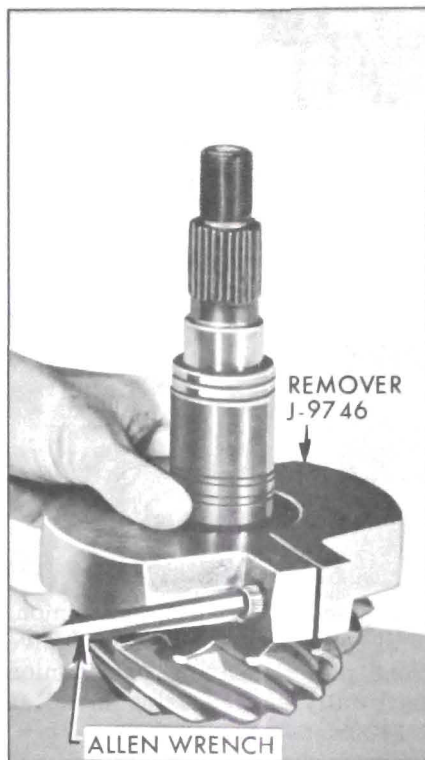
Figure 6-17—Installing Pinion Bearing Remover
