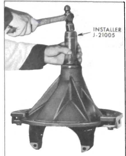
Figure 6-23—Installing Pinion Seal
