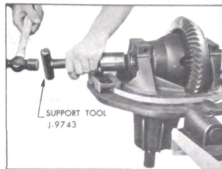
Figure 6-35—Installing Differential Bearing Supports
