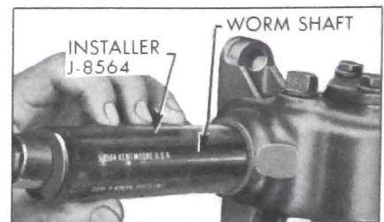
Figure 8-12—Installing Worm Shaft Seal
