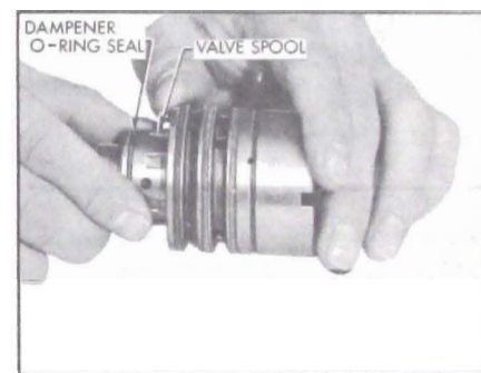
Figure 8-41—Withdrawing Valve From Valve Body
