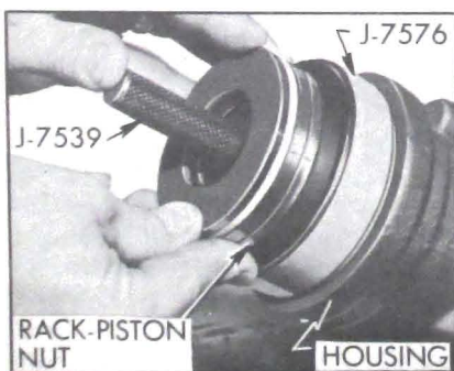
Figure 8-58—Installing Rack-Piston Nut
