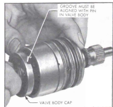
Figure 8-44—Assembling Stub Shaft, Torsion Bar and Cap Assembly in Valve Body
