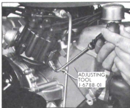
Figure 10-43—Adjusting Contact Point Dwell Angle
