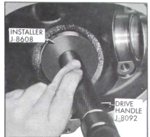
Figure 6-22—Installing Rear Pinion Bearing Outer Race
