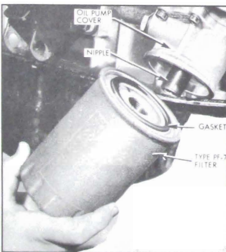
Figure 1-4—Oil Filter Installation
