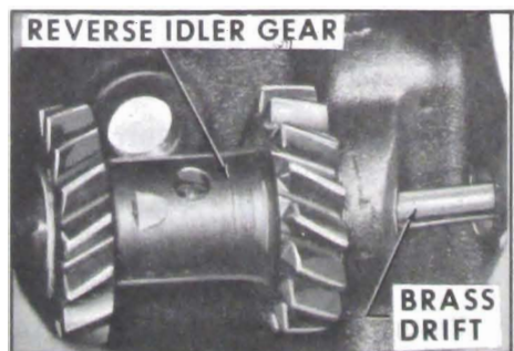
Figure 4-17—Idler Shaft Removal
