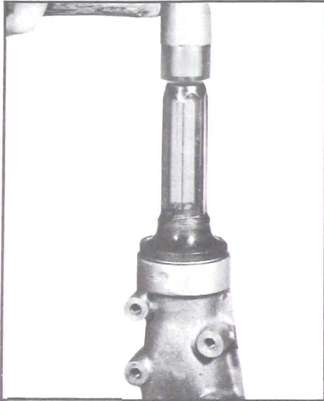
Figure 4-67—Installing Extension Oil Seal
