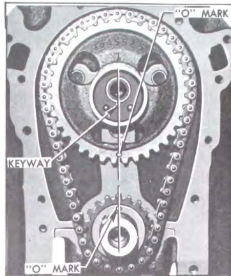
Figure 2-35—Timing Chain and Sprockets Properly Installed
