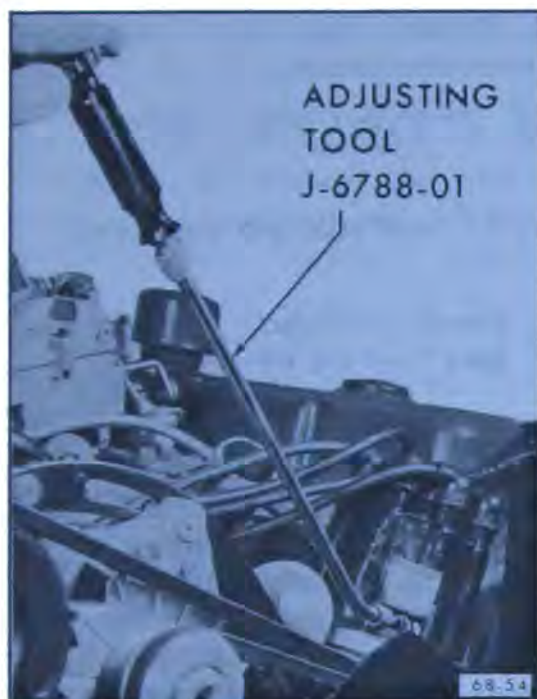
Figure 68-36—Adjusting Contact Point Dwell Angle - V-8 Engines
