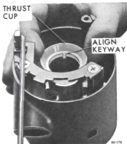
Figure 90-113 Removing or Installing Thrust Cup
